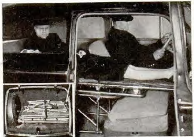
Stretcher rack for sedan folds for loading into trunk, inset
